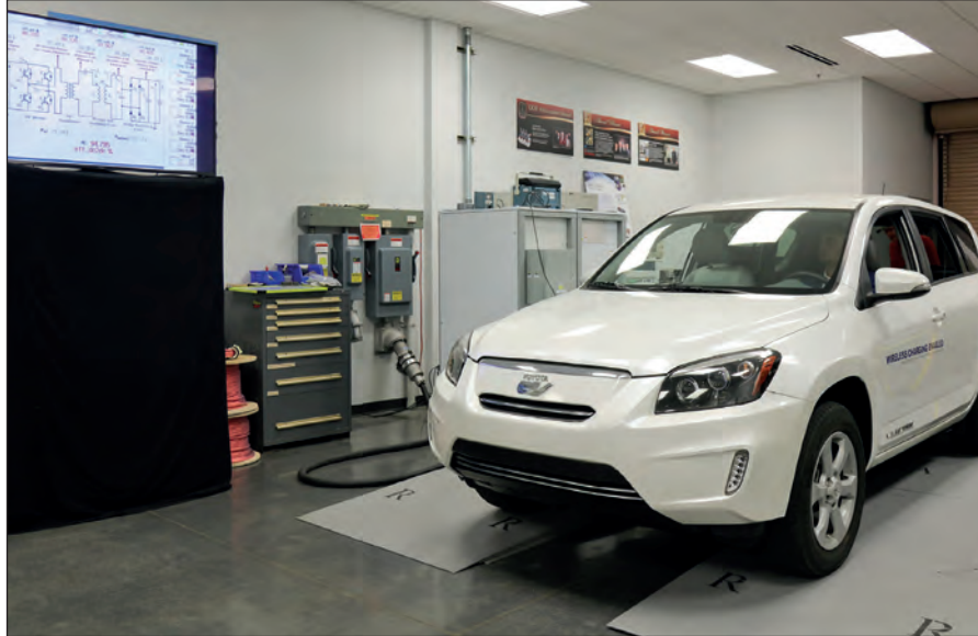
Figure 1. An EV test platform at ORNL that was used to evaluate power modules for wireless charging
